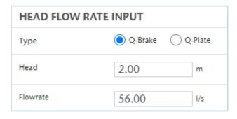
Radio buttons allow the selection of either Q-Brake (Vortex Flow Control) or Q-Plate (orifice plate). This selection can be changed at any time.
